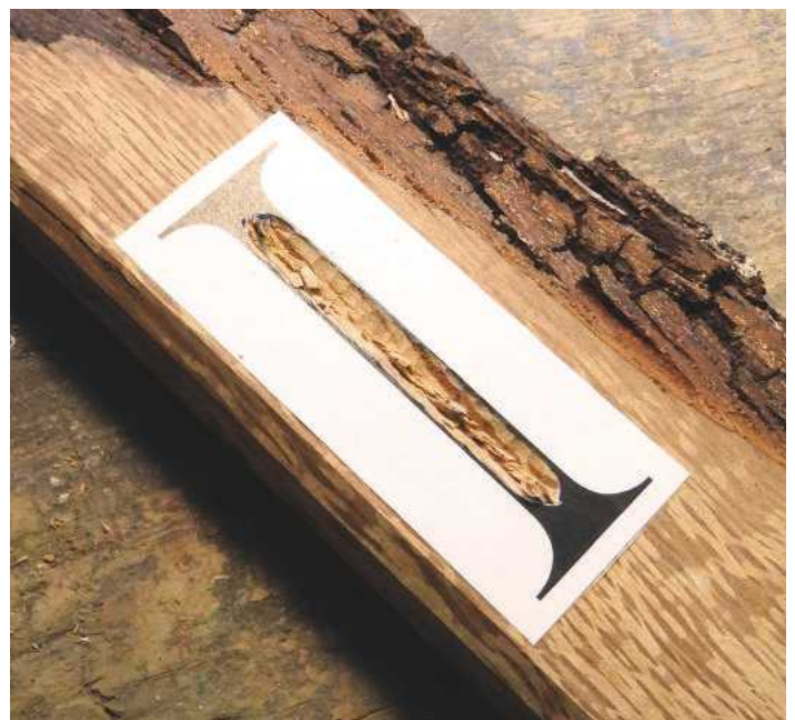
Gouging from either side, not worrying too much about the valley bottom. Edging back to the lines but keeping clear of the serifs
